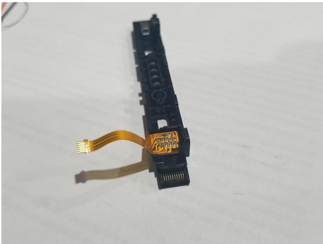
***(Image 15 - JoyCon Slide Connector Board Fully Removed)***
