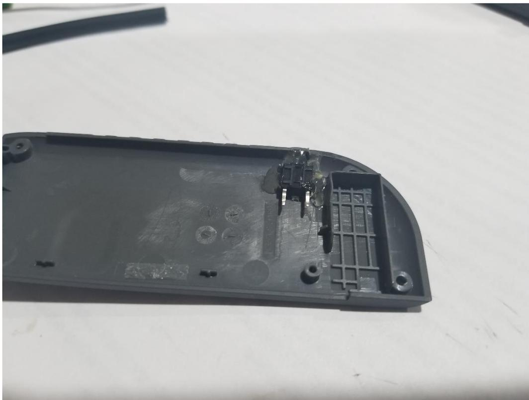
*(Image 18 - Momentary Switch Secured with Hot Glue)*
